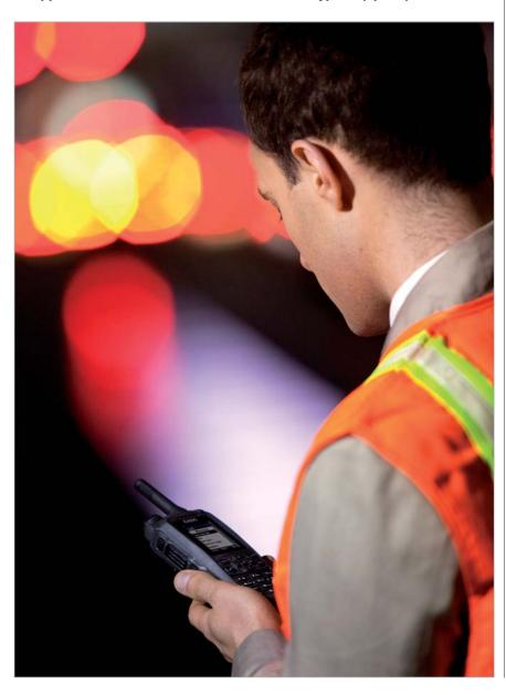
The THR9i TETRA handheld radio from CASSIDIAN® delivers high performance and usability for mission-critical voice and data communication. With IP65 protection, the largest sharpest on the market QVGA display and high battery autonomy the THR9i is a solid and easy to use communication tool.
