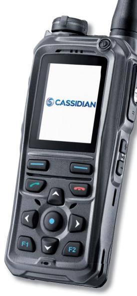
In addition, two freely programmable function keys, F1 and F2, can be assigned to the functions most often needed. The THR9+ also has the fast menu familiar from other CASSIDIAN® TETRA radios. Together with the voice feedback, this makes it possible to use the radio without looking, which is an important benefit when focusing on the task at hand.
